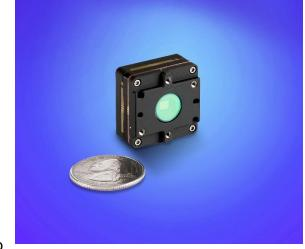
competing shortwave infrared imagers. The lightweight (only 23 g without lens) SWIR camera captures snapshot imagery utilizing a high-performance InGaAs detector with an extremely small 5-micron pixel pitch that enables a short focal-length optic.
