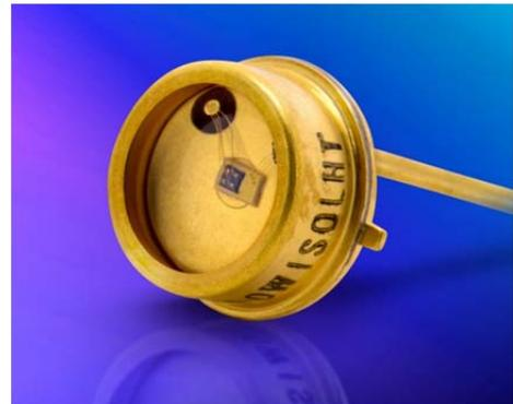
Opto Diode's OD-110WISOLHT features a continuous forward current of 500 mA, power dissipation at 1000 mW and peak forward current of 1.5 A while the reverse voltage is 5 volts. The lead soldering temperature (at 1/16" from the case for 10 seconds) is 260 degrees C. Storage and operating temperatures range from -65 °C to 150 °C with a maximum junction temperature of 150 °C.
