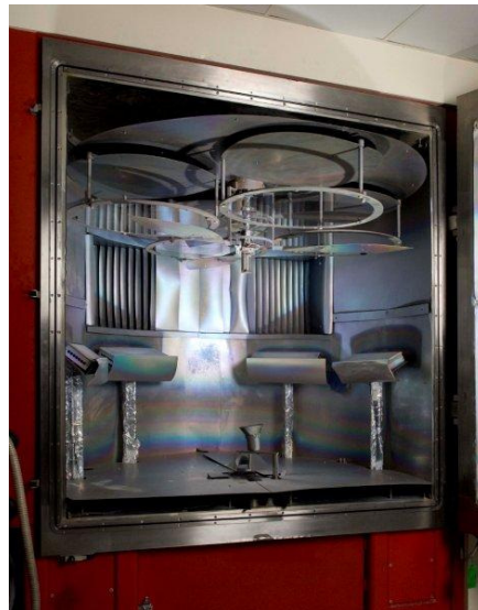
Figure 2 – Large volume, thin film coating chamber.
