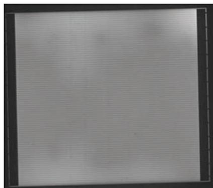
Figure 1. This electroluminescence image of a multi-junction cell was acquired with an InGaAs 1024-pixel line-scan camera array without filtering. The image was cropped to 880 columns  $\times$  773 rows. The horizontal line pattern consists of 10- $\mu$ m lines on 100- $\mu$ m centers.
