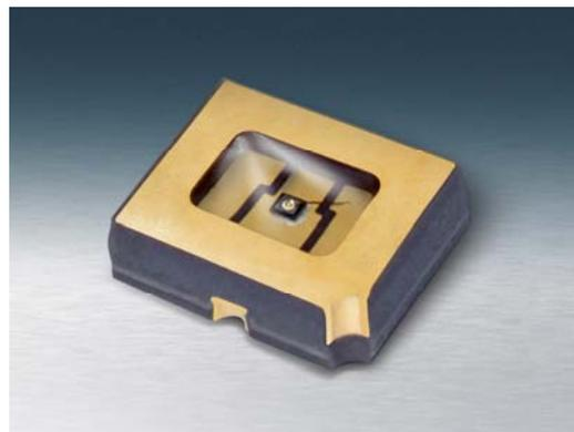
The rugged new surface-mount device is fully operational within a very wide temperature range from -40 °C to +125 °C, making it ideal for use in harsh environmental conditions. The forward voltage of the OD-685C is typically 1.8V with a maximum of 2.2V. The spectral bandwidth at 50 percent is 30 nm. For higher optical power the device may be operated with total power dissipation at 110 mW and continuous forward current at 50 mA or with the peak forward current (at 10µSec @ 300 Hz) at 100 mA.
