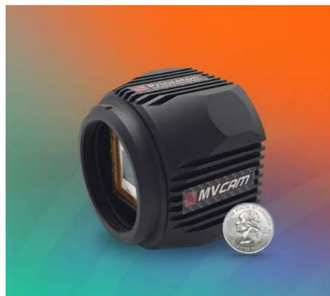
MVCam's advanced digital array (PIRT1280A1-12) generates 14-bit digital image data with no image lag and read noise less than 45 e<sup>-</sup>, which is lower than all other industrial SWIR cameras. The camera uses Medium configuration Camera Link to output the video imagery at the full data rate of 95 fps. Base Camera Link can also be used at lower frame rates. Princeton Infrared Technologies' MVCam is ideal for high-resolution machine vision and microscopy applications.
