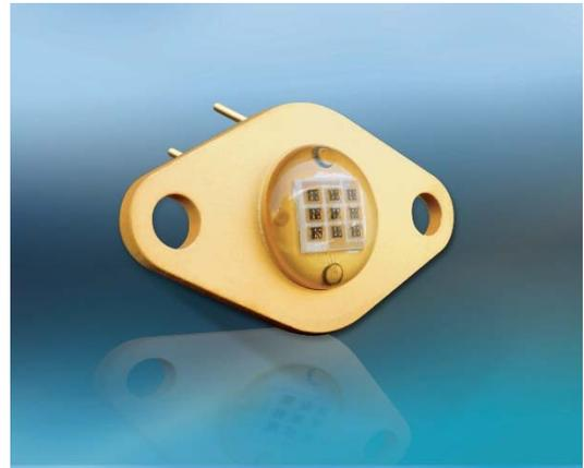
Total power output ranges from 390 mW (minimum) to 500 mW (typical) under test conditions at 300 mA. The spectral bandwidth at 50% is 80 nm, and the half intensity beam angle is typically 120 degrees. The forward voltage of the OD-669 ranges from 13.5 volts (typical) to 15 volts (maximum); reverse breakdown voltage is at minimum 5 volts and 30 volts (typical). Capacitance is 11 pF; the rise time and fall time is typically 3  $\mu$ sec.
