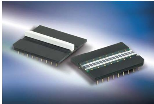
For X-ray or gamma-ray applications, there are three scintillator-mounting options: bismuth germinate (BGO), cadmium tungstate ( $\text{CdWO}_4$ ) and caesium or cesium iodide (CsI). When coupled with a scintillator, the OSI's silicon detector arrays map any medium- or high-radiation energy over to the visible spectrum via scattering effect. For larger-scale assembly, multiple arrays may be installed to achieve optimum results.
