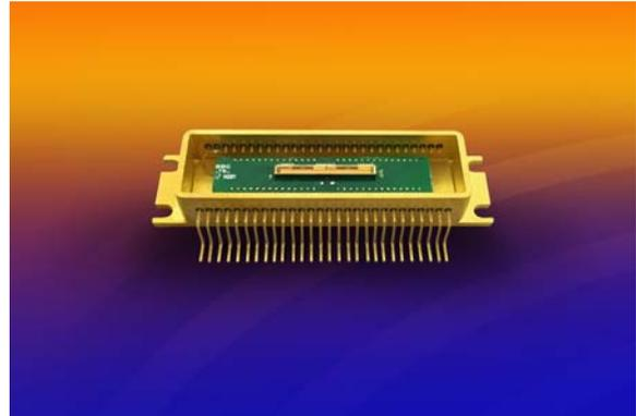
The 1024L1 uses a single digital ROIC chip to minimize variation from output to output, which is often an unwanted feature on linear arrays with multiple ROICs. The chips have built-in 14-bit analog-to-digital converters that maximize dynamic range (>6000:1) and minimize noise, while delivering 34klines/s at 1024 elements. It also has the largest selection of full wells, from 75ke- to 100Me-, in the industry.
