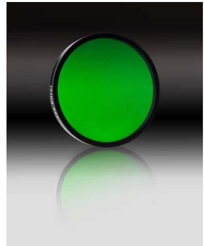
These ultra-steep filters with >OD6 blocking out of the band and state-of-the-art center wavelength tolerances of  $< \pm 0.3\%$  offer the highest transmission levels available with a passband average of >95% (see graphic). The new filters aid in the fluorescent detection of the virus and cover most common fluorophores for single and multiplexed qPCR filters, including FAM, Cy5, HEX, JOE, ROX, TexasRed®, and TRITC.
