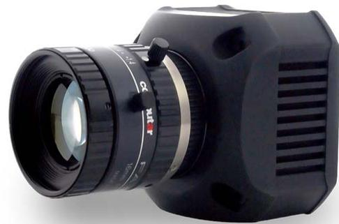
The new InGaAs photodiode array features a patented readout integrated circuit (ROIC). Available in 640 x 512 (with 15-micron pitch) or 320 x 256 (with 25-micron pitch) pixel resolution; both operate in the SWIR spectrum from 900 nm up to 1700 nm with high quantum efficiency. Power consumption is less than 1.5W. By design, the proprietary NIT ROIC has proven to be highly functional for fast, triggered imaging applications such as range-gated imaging and synchronous illuminated imaging.
