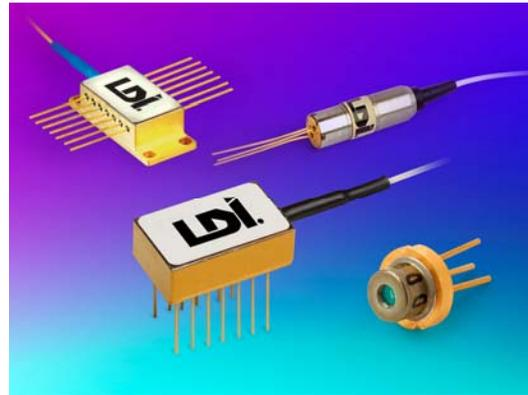
or 3-pin TO56 housings. RoHS compliant, the high-peak pulsed laser diode modules operate typically at a center wavelength of 1490 nm (1470 nm, min. to 1510 nm, max.). They deliver no less than 100 mW optical power (fiber) and a minimum of 300 mW (TO56).
