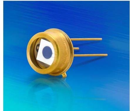
Electro-optical characteristics include responsivity at 0.09 A/W (minimum) to 0.115 A/W (typical) and dark current of 1nA. The reverse breakdown voltage ranges from 25 V (minimum) to 50 V (typical), and capacitance is 500 pF (minimum) to 1500 pF (maximum). Response time is 1  $\mu$ s (minimum) to 2  $\mu$ s (maximum).
