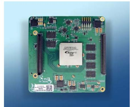
The A10 board supports both OpenCL™ and high-level synthesis (HLS) tools for accelerating design cycles and targeting C/C++ code to the FPGA. Critical Link's innovative MitySOM-A10S-DSC processor with embedded Linux provides operating system support, versatility, and ease of customization for complex imaging platforms.
