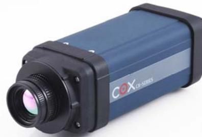
Well suited for a variety of radiometric imaging tasks, the CX640 features onboard thermography capabilities with on-screen display of temperature data points presented on the NTSC/PAL analog video signal. Radiometric measurements range from -20° C to 650° C. Communication to the camera is achieved via either RS-485 or Ethernet with the camera displaying temperature information of up to ten spots, as well as two user-defined regions-of-interest (ROIs) with temperature triggered hardware alarms.
