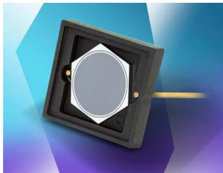
The AXUV20A photodiode shunt resistance is 100 MOhm, minimum. Reverse breakdown voltage is 5 volts, minimum, and 10 volts, typically. Other features include capacitance at 4 nF, typically, with a maximum of 10 nF, and a rise time of 2 µsec. The AXUV series of photodiodes exhibits response to electron energy levels as low as 100eV. To view typical AXUV20A response graphs, see pg. 2 of the data sheet here: <https://optodiode.com/pdf/AXUV20ADS.pdf>.
