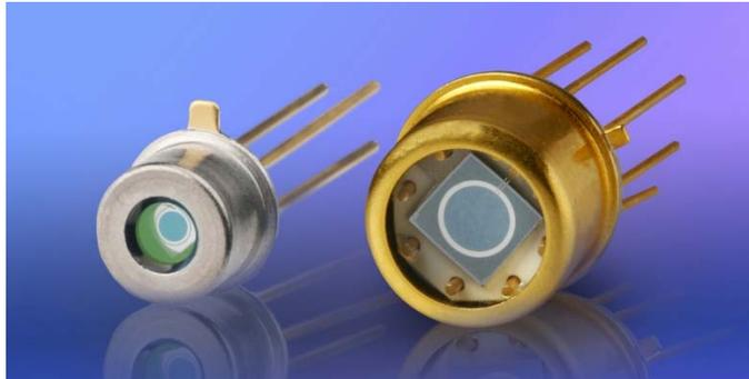
APX's 400-1700 nm PSD features 2k $\Omega$  inter-electrode resistance, high shunt resistance, low capacitance, and 20  $\mu$ m position detection error. The highly sensitive PSDs are conveniently housed in a hermetically sealed TO-5 package or a 5 mm by 3.6 mm surface mount ceramic package with an anti-reflective window, making them suitable for integration into a variety of systems.
