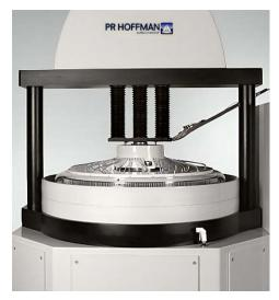
such as Fused Silica, BK-7, and other materials. The machine balances internal stresses within materials, minimizing the risks of warping or deformation for optimal consistency and repeatability on substrates up to 250 mm diameter.
