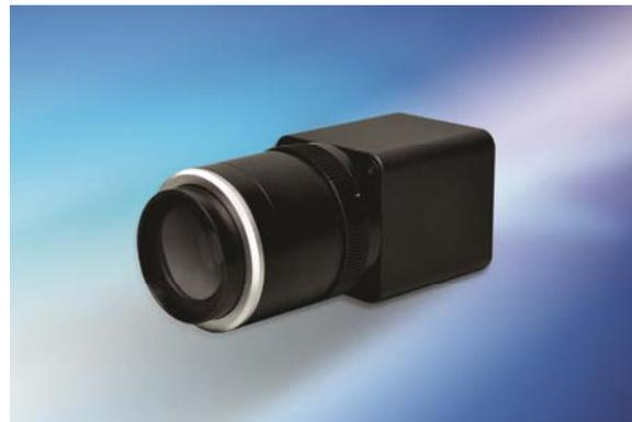
Lightweight (less than 120 g without lens), compact (less than 4.5 in<sup>3</sup>), and low-power (less than 3.8 W at 20 degrees C), the GA1280JSX OEM model can be easily integrated into unmanned aircraft systems (UAS) or other handheld, mobile, and/or robotic systems. It operates optimally in moonlight to daylight and images through dust, fog, and smoke. It is also capable of multi-laser spotting and tracking and covert surveillance with passive 24 hour/7day operation.
