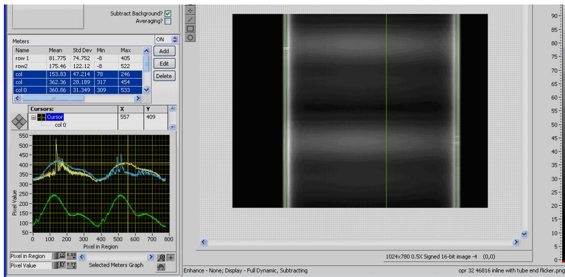
**Figure 3:** Capturing the lamp output variation over the power line cycle.
