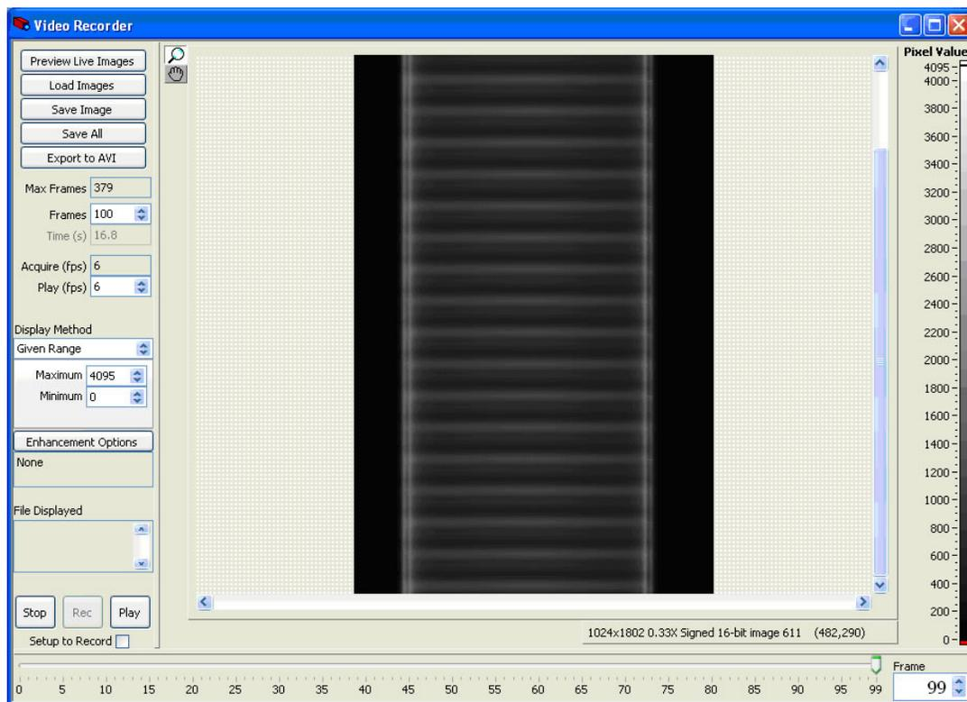
**Figure 6a:** Video recorder screen showing last frame of 100 frame video, capturing 20 cycles of the 120 Hz light pulses from office fluorescent lamps.
