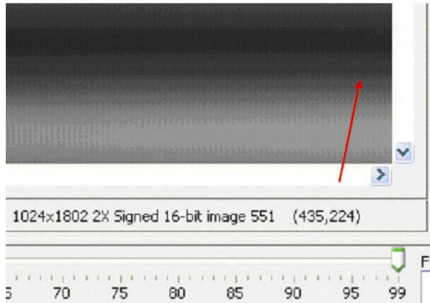
**Figure 6d:** Cursor intensity is 552 counts and its position is at (X,Y) position (435,224). The red arrow points to the dark feature used to gauge image position drift from frame 0 to frame 99.
