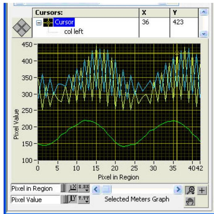
**Figure 9:** Expansion of first 42 lines captured from the high-efficiency lamps, showing very high frequency pulses from the tube ends and a 4,600 ripple frequency for the phosphor output.
