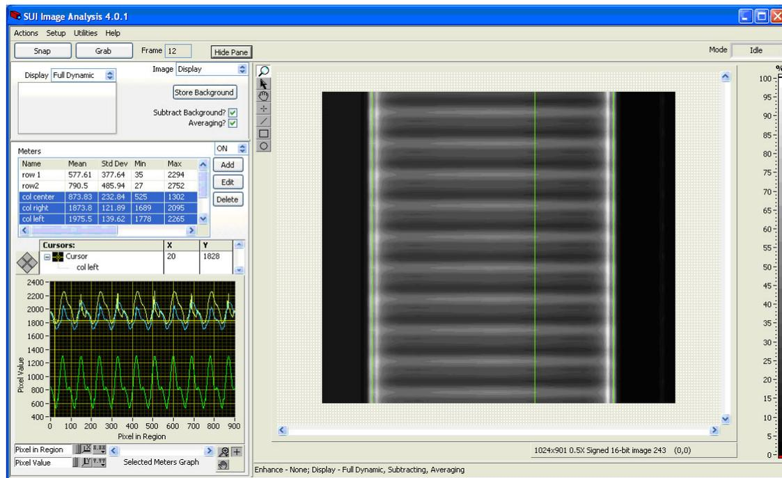
**Figure 5:** Measuring the power line frequency and camera line rate in a single frame.
