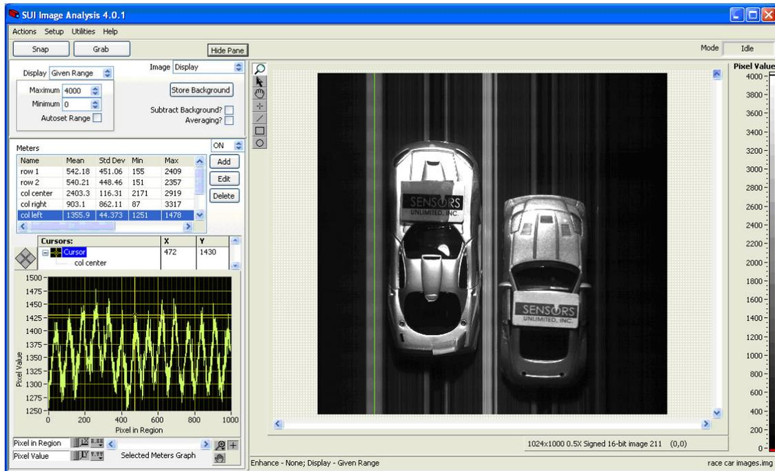
**Figure 1:** Incandescent lamp ripple — the vertical green cursor visible on the above image to the left of the cars and the associated line profile graph on the left shows the ripple riding on top of the incandescent lamp illuminating the scene.
