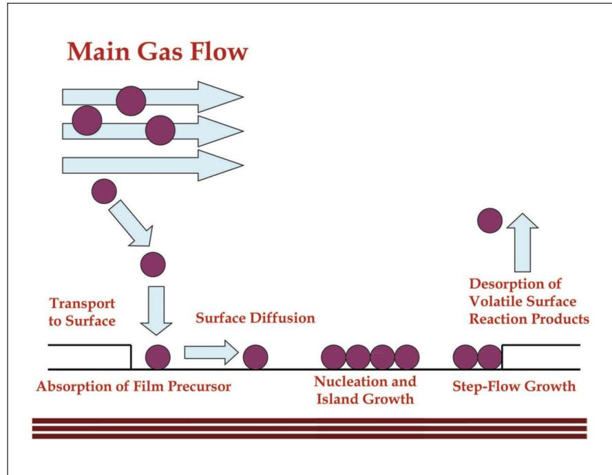
Figure 2. Schematic of film growth mechanism by CVD.
