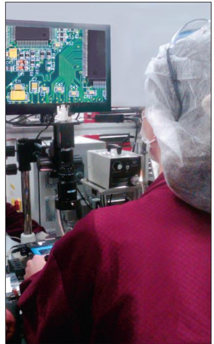
Figure 2. Circuit board inspection line utilizing the new HD-210D imaging system.
