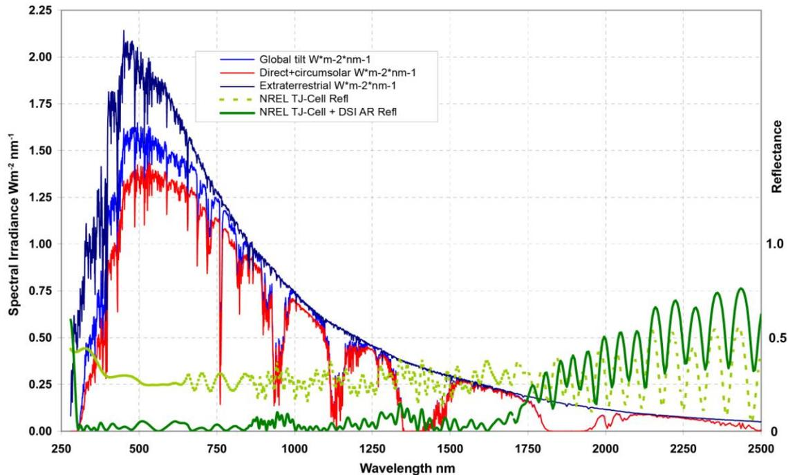
**Figure 2:** Uncoated and coated specular reflectance of LM triple-junction solar cell overlaid with ASTM G173-03 Solar Spectra.
