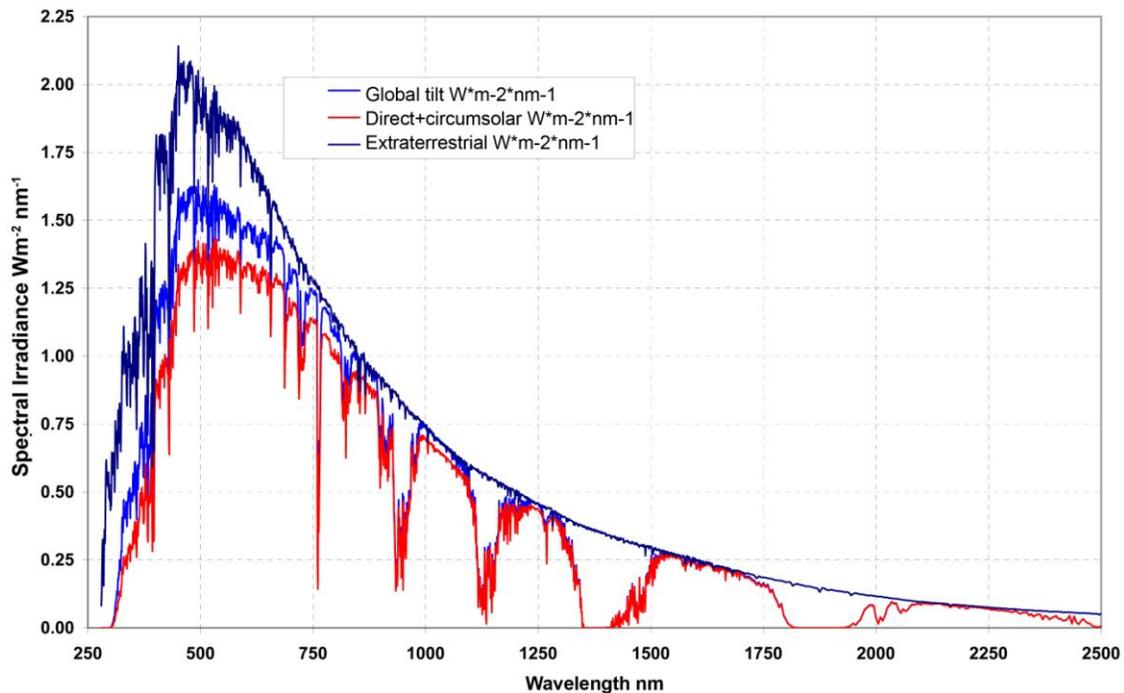
Figure 1: ASTM G173-03 solar spectra
