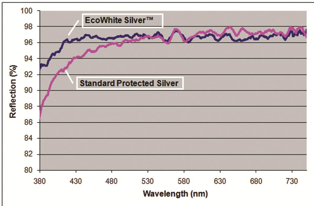
**Figure 3:** The reduction in blue roll-off using EcoWhite Silver coatings, as compared to standard protected silver coatings, saves material, reduces costs and results in better performance.
