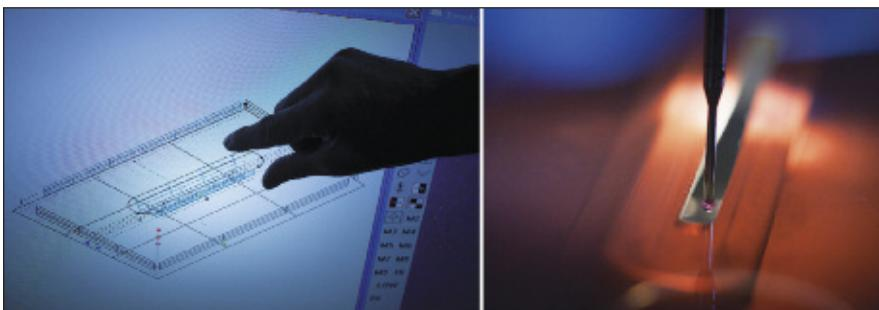
Figure 2. After machining, all dimensions are verified using a Starrett computer measurement machine (CMM) equipped with a touch probe that measures parts to within 2 microns.
