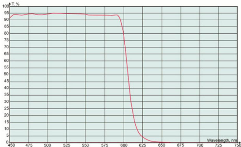
**Figure 2: Typical results from coating, measured on PG&O's Perkin Elmer Lambda 950**
